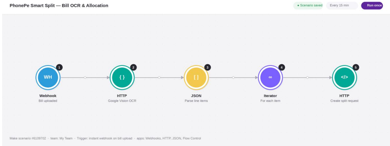
Figure 4.3 — Backend: Make scenario #6109702. Webhook → HTTP OCR → JSON parse → Iterator (per item) → HTTP create split request.
